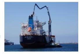
articulated hydraulic boom mounted on top of a tower. The end of the ducting uses high temperature flexible piping to connect to the generator and/or auxiliary boiler exhaust on the vessel. Once connected a slight suction is used to capture the vessel exhaust. This exhaust moves through the capture and treatment system where it is scrubbed of NOx, PM, and SOx, and re-enters the atmosphere cleaner than the ambient air.
