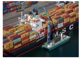
for over a thousand hours of commercial use. During these operations, there has never been an incident that posed a threat to the vessel, its equipment, the port, or the environment. Additionally, an independent third party analysis has determined that in ports that have no shore power infrastructure AMECS obtains an equivalent air emissions reduction at one third the total cost of shore power.
