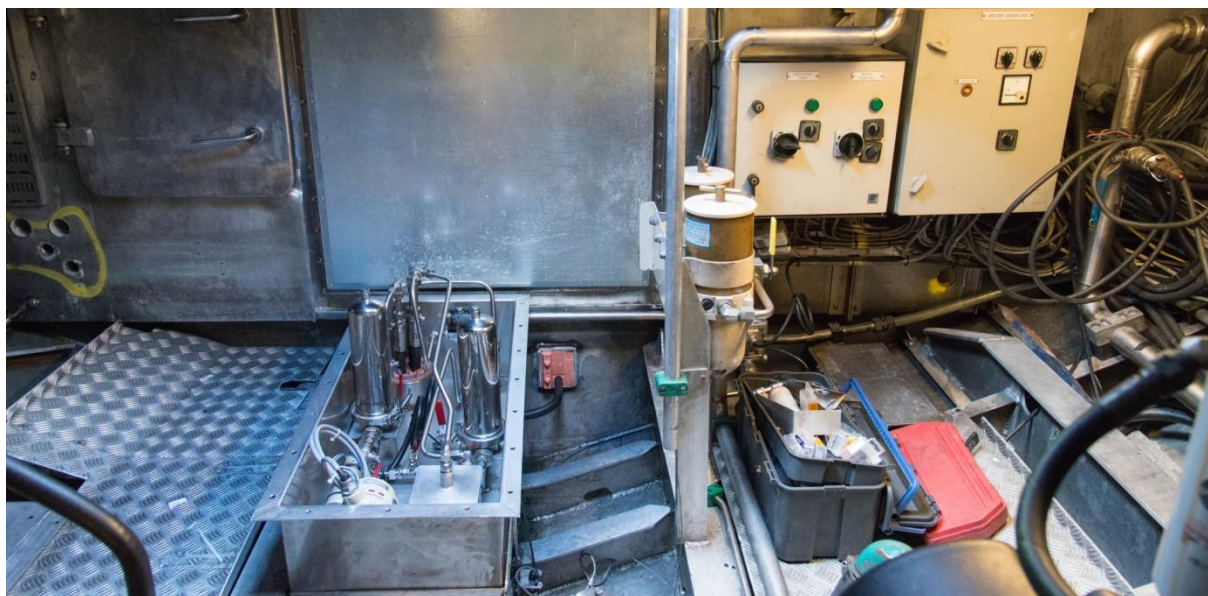
Figure 2-7: Photo of the open pump chest, looking forward in the engine room. Piping and fuel filters are visible, with the intermediate catch tank visible along the vapour detector closest to the camera. Double walled pipes can be seen entering the pump chest furthest away from the camera, and entering the tank room below to the right of the pump chest.
