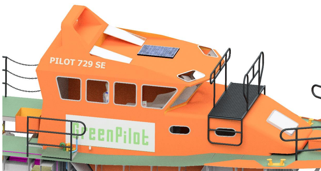
Figure 6-3. Illustration of the solar panels mounted on the cabin roof.
