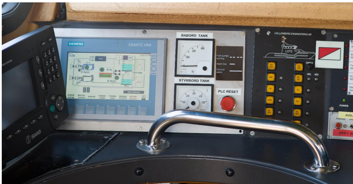
Figure 2-11: The HMI panel at the steering position.
