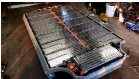
Figure 7-2. Tesla Model S battery. The battery cells and cooling are built in to the chassis.
